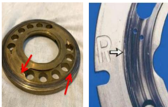
Gambar 8. Terdapat abrasive wear port plate, not use again
