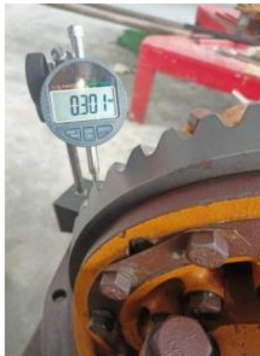
Gambar 10. Proses pengukuran backlash
