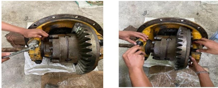
Gambar 3. Proses pembongkaran komponen differential baut bearing caps
